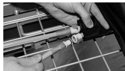
C. Using the quick connectors, connect the air inflation hoses to the air cell hoses - 'Red to Red' - ensuring the hoses are not twisted or kinked.
